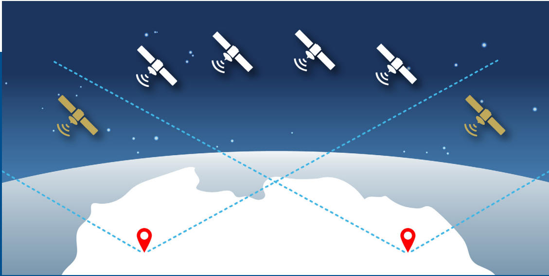
Figure 1. SkyWire™ technology leverage signals from GNSS satellites that are simultaneously visible (in common view) to at least two ground locations.
