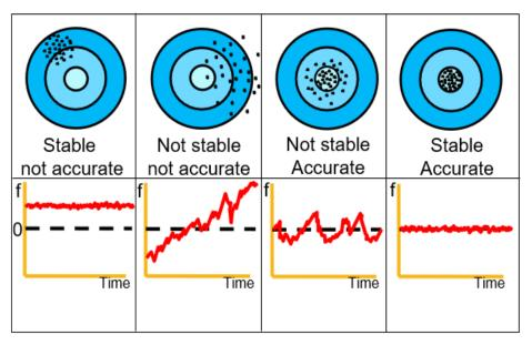
Samples of measurements of time-error or frequency offset
