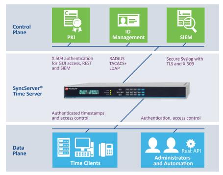
traffic between ports; each port has access control lists, and all ports can have unique network configurations. Management access is strictly limited to a single LAN port for further isolation from the network.
