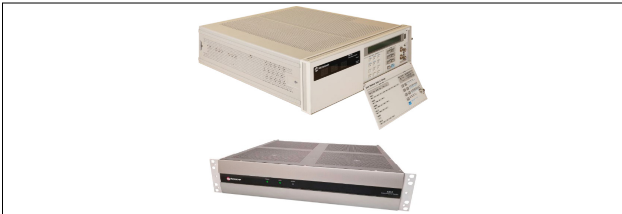
FIGURE 9: Microchip 5071A and 4310B Cesium References.
