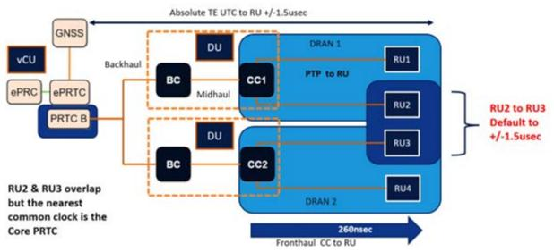
The impact of the timing error goes beyond the radio with time error out of the budget as this will result in interference with adjacent radios. Therefore, the extent of damage from the phase sync timing error is considerably greater than the source node.
