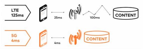
Precise synchronization is directly linked to the system latency, because with the reduced size of the guard bands, we have an improvement in performance. Timing is also important in the formation and direction of 5G radio beams. When an instruction is sent from a centralized server to a certain radio, in order to concentrate more or less bandwidth for an user, this instruction must be executed immediately.
