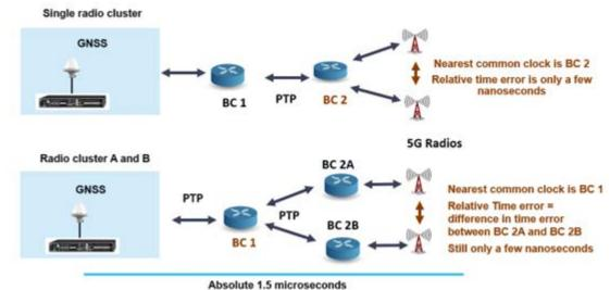
2. Implementation scenarios using only GNSS at cell sites (GNSS everywhere) technically wouldn't work, because the typical phase error of those devices (embedded GNSS) are around 400 ns, which in itself is much higher than what 3GPP standard specifies for fronthaul and is outside the relative time error specifications.
