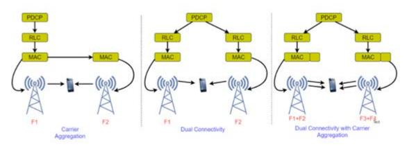
For this technology, 3GPP requires a maximum relative time error between radios of 130 ns (FR1) or 260 ns (mmWaves) (FR2). Due to this extremely restricted numbers, the 3GPP also recommends the use of network based PTP (G.8275.1 protocol) timing services with full-on path support (boundary clocks) as:
