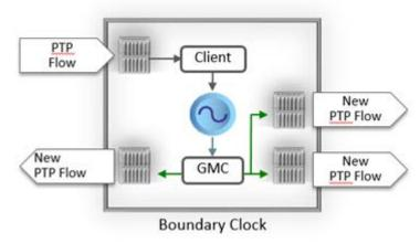
In a full-on path support architecture, based on ITU-T G.8275.1 all T-BC switches now are part of the PTP transport as common clock to the final client destination the radio unit.
