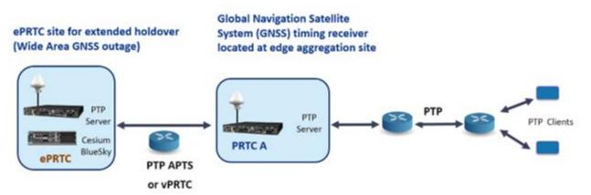
In a use case where the operator uses the Microchip TP4100 GNSS PRTC source clock GMC with a Rubidium holdover oscillator that will guarantee UTC alignment for a long period (43 hours), a GNSS disruption or failure will not impact overlapping radios or radio clusters that are receiving their network-based PTP timing services from a different GNSS PRTC source clock.
