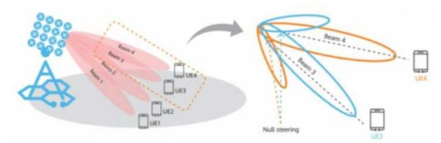
To increase the resilience (Signal-to-Noise Ratio, or SNR) of a transmitted signal and channel capacity, without increasing spectrum usage, a common frequency can be steered simultaneously in multiple directions. We are now applying the MIMO concept.
