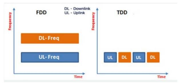
Guard bands are implemented to ensure that there is no overlap in the timeslots transmitting and receiving information, otherwise the frequency overlaps and causes interference between adjacent timeslot channels.
