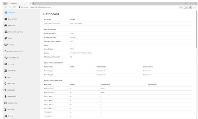
The CMT can be accessed by establishing a connection to the device's administrator (admin) USB-C<sup>®</sup> port or its administrator (admin) Ethernet port. This process is described in 9.1. Establishing a Connection to the GridTime 3000. Once a connection has been established, an admin port IP address can be typed into a web browser on your PC, and the login screen for the CMT will appear.
