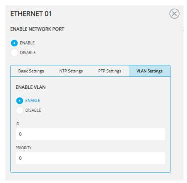
Once enabled, VLAN tags will be applied to all outgoing traffic from the port including NTP and PTP.
