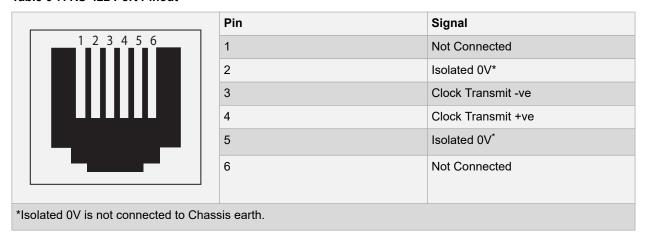
An RJ-12 to male DB9 cable accessory is optionally sold with the GridTime 3000, which can be used to interface the RJ-12 ports with a female DB9 connector.
