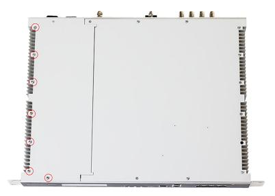
2. Remove the power supply bay lid compartment, shown below.
