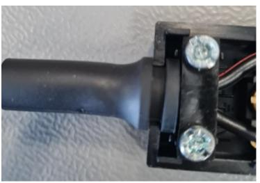
8. Clip the second half of the housing in place and fasten the screw.
