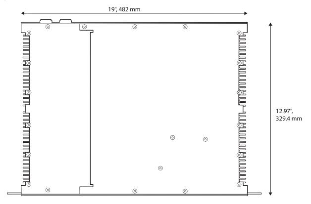
The case's lid is comprised of two segments — the main compartment, and the power supply bay.
