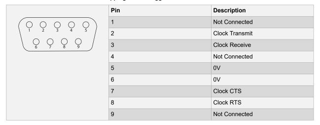
Table 6-9. RJ-12 to DB9 Cable Pin Mapping When Plugged Into RS-422 Port
