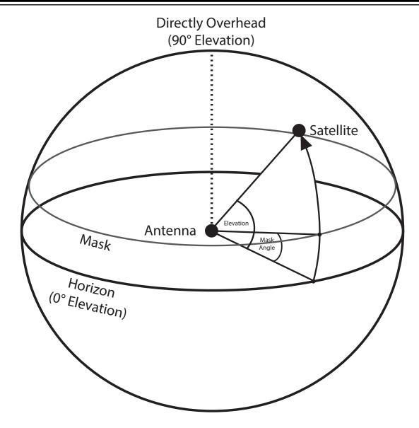
Signals from satellites that are obstructed by objects on the horizon such as mountains may provide inconsistent GNSS coverage due to interference. The mask angle threshold setting provides a method to filter out these inconsistent signals ensuring the GridTime 3000 only uses stable and accessible satellites.
