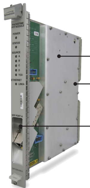
PTP Cards for the SSU 2000/SSU 2000e. Optional SyncE capability.
