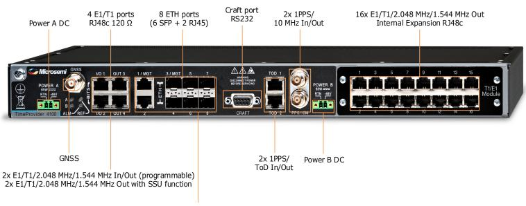
1x packet Ethernet In + management (with SyncE) - 1x RJ45 or 1x SFP cage. Either in-band management or out-of-band. 6x packet Ethernet Out (with SyncE) - 1x RJ45 and 5x SFP cage.
